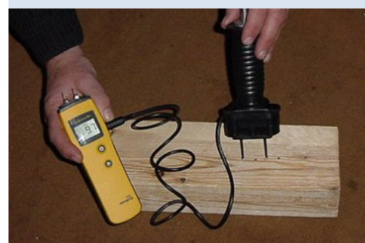
Moisture meter reading.
