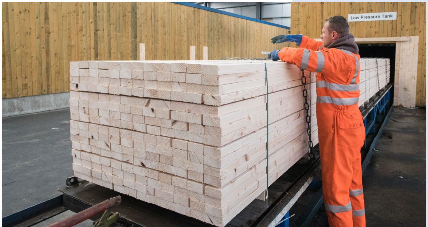
A typical wood preservative pressure treatment plant. Photo courtesy of BSW Timber.
