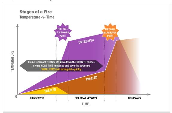
Flame retardant treatment will enhance the **reaction to fire** properties of wood-based materials, reducing ignitability and consequent spread of flame. Slowing down the development of the fire and allowing significantly more time for the occupants of a building to escape and for the fire to be extinguished.
