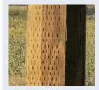
penetration requirement (even for permeable species such as pine). Mechanical incising of the surface is now used widely to help achieve the desired penetration.
