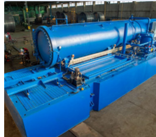
A pressure treatment vessel under construction. Photo courtesy of Tweddle Engineering.
