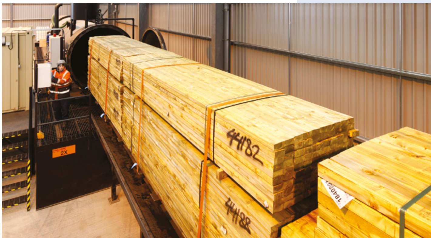
A typical wood preservative pressure treatment plant. Photo courtesy of Södra.
